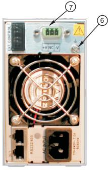
Fig. 4-2: Rear panel connections
