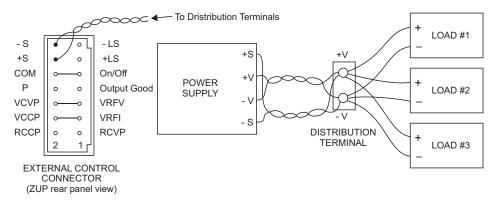
Fig. 3-4: Multiple load connections with distribution terminal
