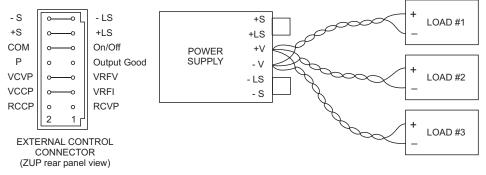
Fig. 3-3: Multiple load connections with distribution terminal
