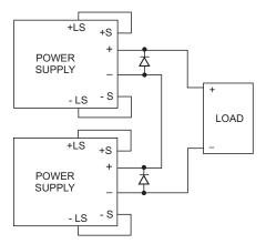
Fig. 4-12: Series connection with local sensing.
