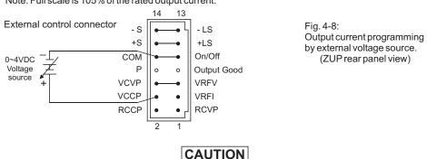
The Com pin at the external control connector is connected to the -Sense potential. NEVER connect the Com pin (pin10) to any potential, as it may damage the power supply.
