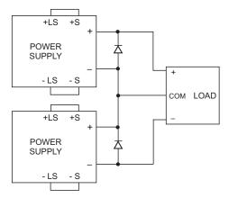
Fig. 4-14: Series connection for bipolar output
