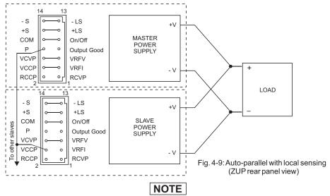
With local sensing it is important to minimize the wire length and resistance. Also the wires resistance should be as close as possible to achieve current balance between power supplies.
