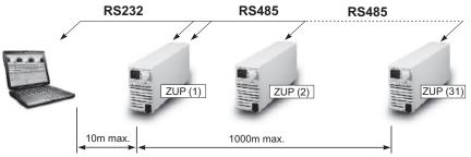
Fig. 5-1: Linking ZUP units with RS232 control.
