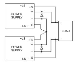
Fig. 4-13: Series connection, remote sensing.
