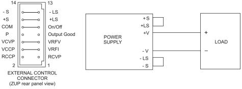
Fig. 3-1: Single load connection, Local Sensing
