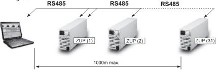
Fig. 5-6: Linking ZUP units to RS485 control.
