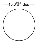
Panel Cutout Dimension Panel thickness = 1 to 4 mm
