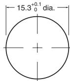
Panel Cutout Dimension Panel thickness = 1 to 4 mm
