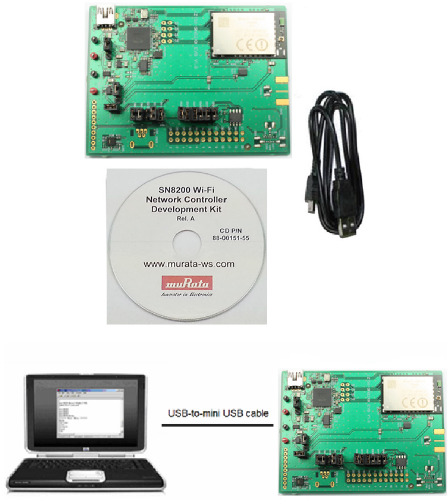
Figure 11 - Typical SN8200 Development Kit
