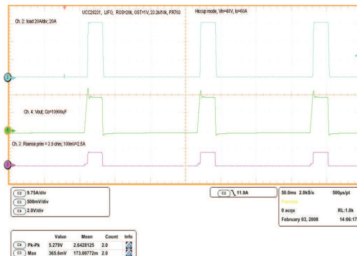
Figure 42. Cycle-by-Cycle Current Limit
