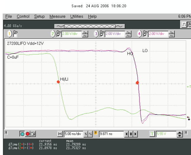
Figure 32. V_{LO} and V_{HO} Falling Edge Delay Matching
