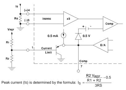
Figure 7. Pulse-by-Pulse Current Limiting
