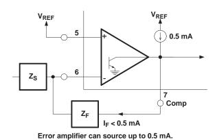
Figure 3. Error-Amplifier Output Configuration
