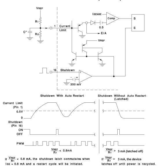
Figure 8. Soft-Start and Shutdown/Restart Functions
