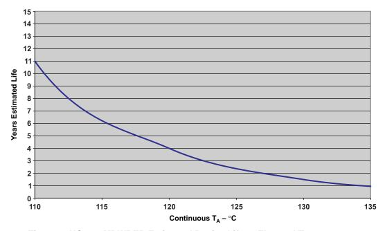
Figure 1. UC1846MDWREP Estimated Device Life at Elevated Temperatures Wirebond Voiding Fail Modes
