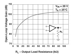
Figure 5. Error-Amplifier Open-Logic DC Gain vs Load Resistance
