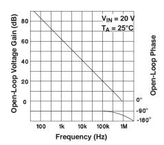
Figure 4. Error-Amplifier Gain and Phase vs Frequency
