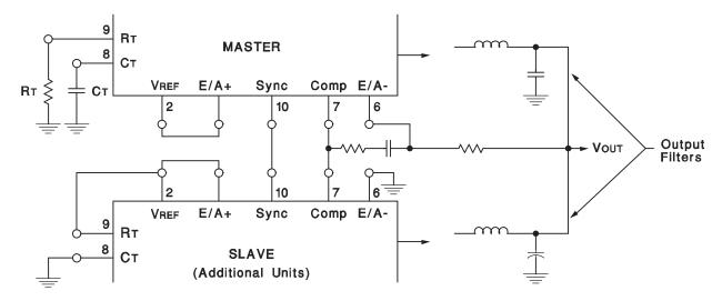
Slaving allows parallel operation of two or more units with equal current sharing.
