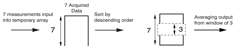
Figure 28. MAV Filter Operation (Patent Pending)
