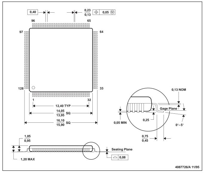
NOTES: A. All linear dimensions are in millimeters. B. This drawing is subject to change without notice.
