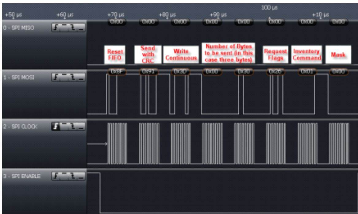
Figure 5-20. Inventory Command Sent From MCU to TRF7970A
