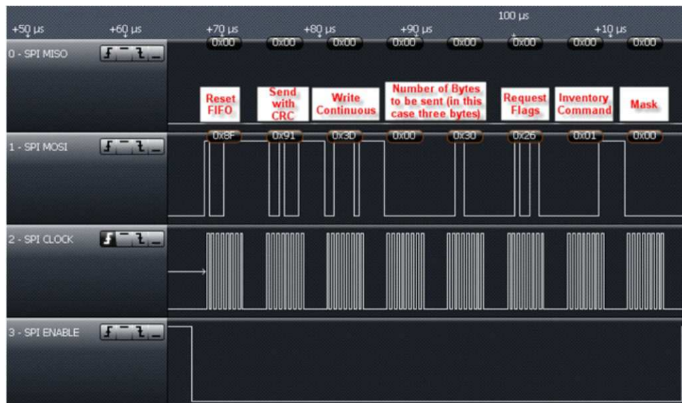
Figure 5-20. Inventory Command Sent From MCU to TRF7960A
