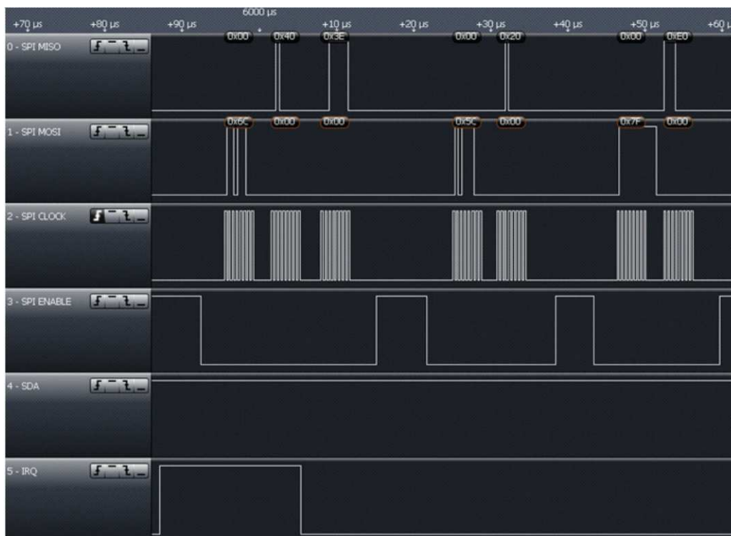
Figure 5-24. IRQ With One Byte in FIFO
