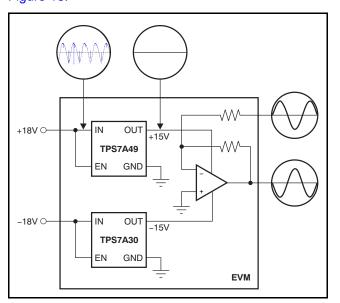
Figure 29. Post DC/DC Converter Regulation to High-Performance Analog Circuitry
