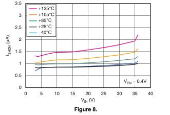
SHUTDOWN CURRENT vs INPUT VOLTAGE
