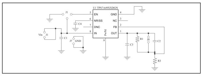
Figure 31. Schematic for PCB Layout Example
