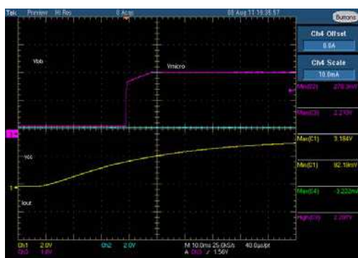
Figure 29. LDO MINI Startup Waveform with VIN Rising Input battery connected to 27Ω resistor and 1000μF capacitor Ch1: VBAT rising. Ch 3: VMICRO (LDO MINI output)
