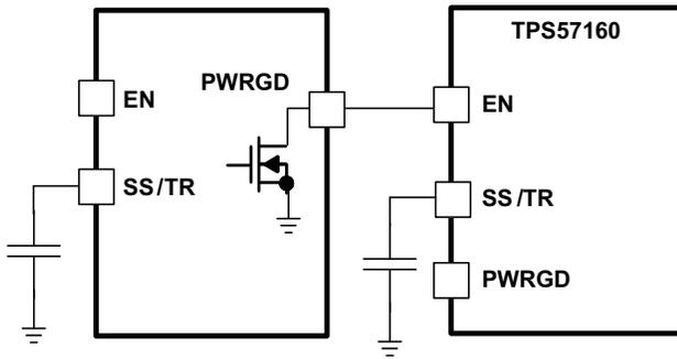
**Figure 32. Schematic for Sequential Startup Sequence**
