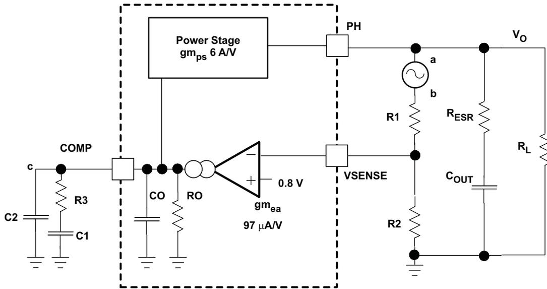
Figure 47. Small Signal Model for Loop Response
