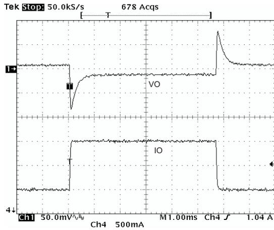
Figure 52. Load Transmit
