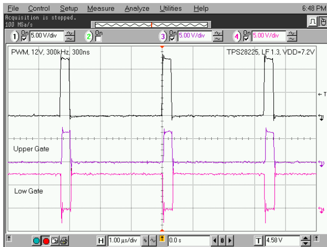
Figure 22. 12-V PWM Pulse at V_{DD} = 7.2 V
