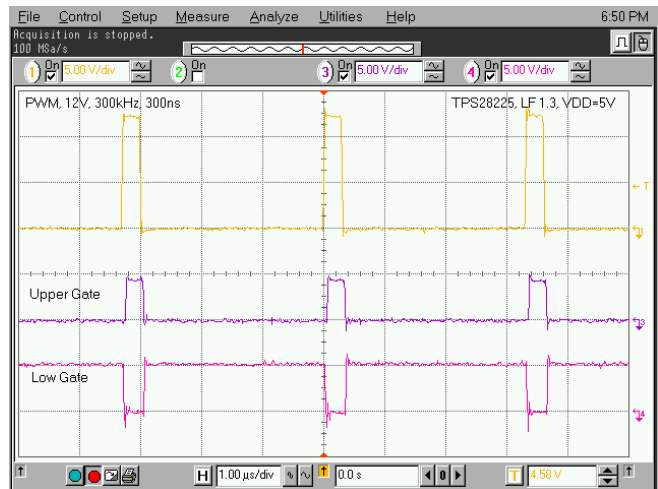
Figure 23. 12-V PWM Pulse at V_{DD} = 5 V
