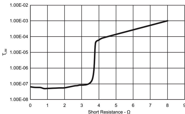
Figure 11. Overcurrent Response Time vs Short Resistance
