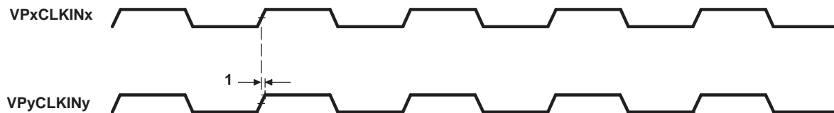
Figure 5-57. Video Port Dual-Display Sync Timing
