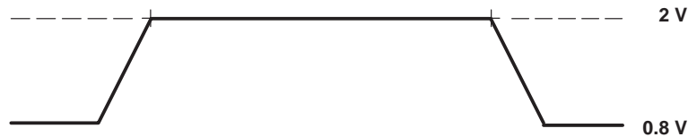
Figure 13. 'C32 Input Levels
