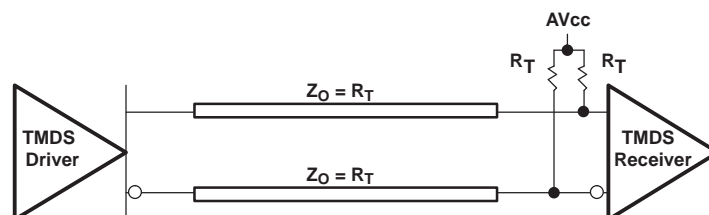
Figure 3. Typical Termination for TMDS Output Driver
