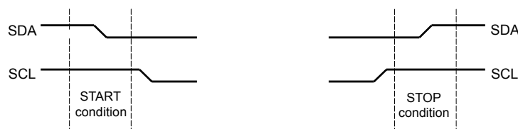
Figure 16-3. START and STOP Conditions
