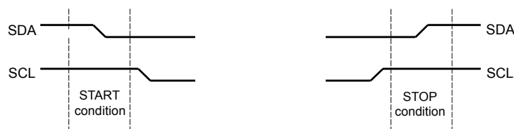
Figure 16-3. START and STOP Conditions
