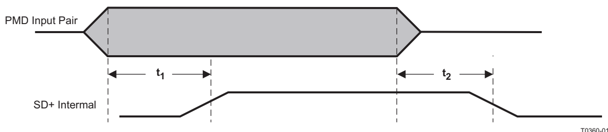
Figure 9-20. 100Base-TX Signal Detect Timing
