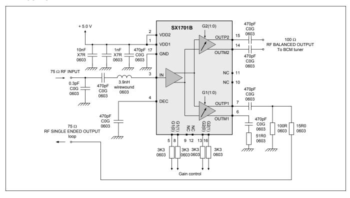
Figure 5. Differential output with loop-through.
