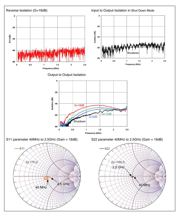
Figure 3. Typical Operating Characteristics Curves.
