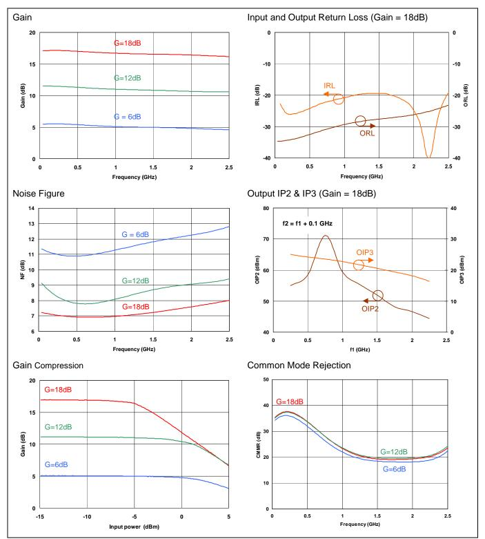
Figure 2. Typical Operating Characteristics Curves.
