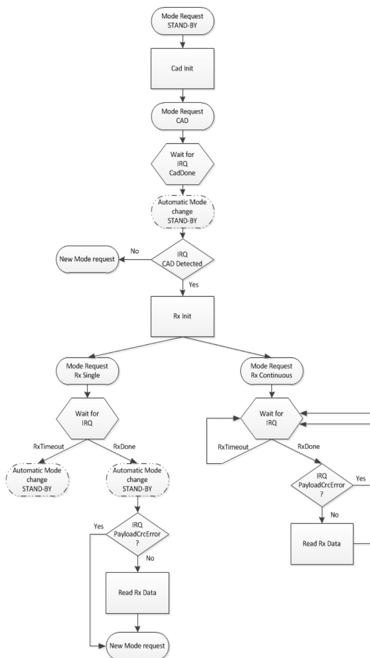
Figure 11. LoRa™ CAD Flow
