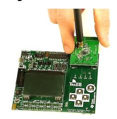
Insert a CC1200EM board into the TrxEB as shown above. Connect the antenna to the SMA connector on the EM.
