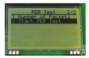
When selecting "Start PER Test", the master (receiver) will begin to count the number of received packets and provide some statistics.
