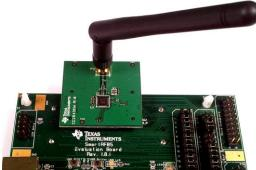
Next, mount the CC2543EMs firmly on to connectors P5 and P6 on the SmartRF05EB.
