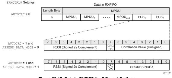
Figure 23-15. Data in RXFIFO for Different Settings
