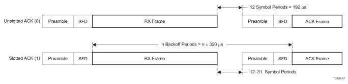
Figure 23-17. Acknowledgment Timing
