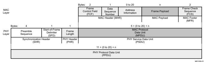
Figure 23-3. Schematic View of the IEEE 802.15.4 Frame Format [1]
