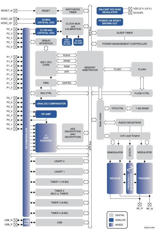
Figure 1-2. CC2540 Block Diagram
