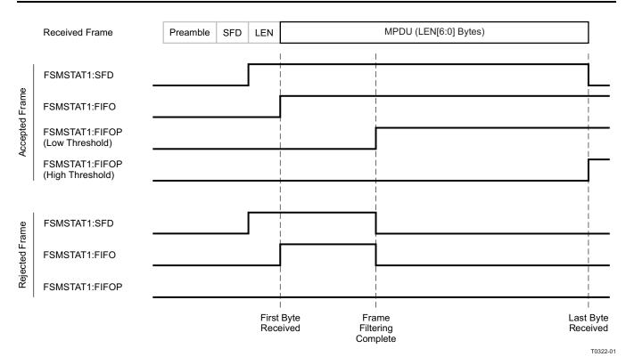
Figure 23-19. Behavior of FIFO and FIFOP Signals
