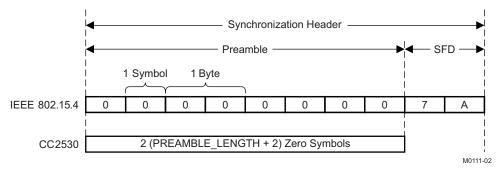
Figure 23-8. Transmitted Synchronization Header
