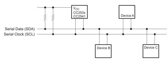
Figure 20-2. I<sup>2</sup>C Bus Connection Diagram
