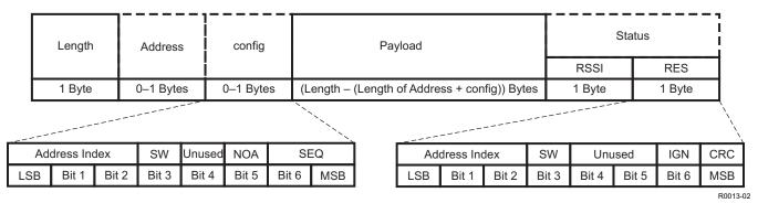
Figure 25-10. Structure of Packets in the Rx FIFO
