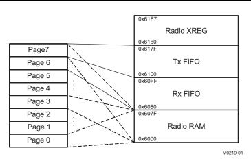
Figure 25-1. Mapping of Radio Memory to MCU XDATA Memory Space
