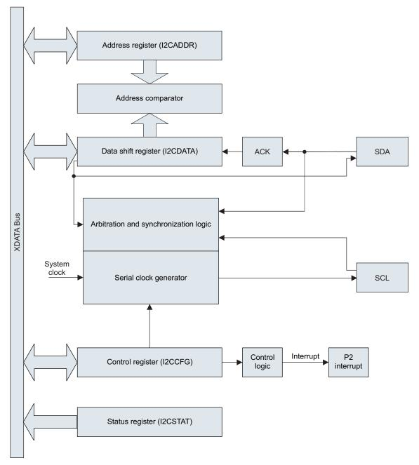
Figure 20-1. Block Diagram of the I<sup>2</sup>C Module
