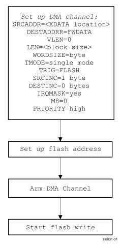
Figure 6-1. Flash Write Using DMA
