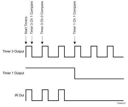
Figure 9-8. Modulated Waveform Example
