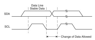
Figure 20-4. Bit Transfer on I<sup>2</sup>C Bus
