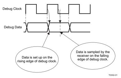
Figure 3-1. External Debug Interface Timing
