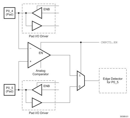
Figure 19-1. Analog Comparator
