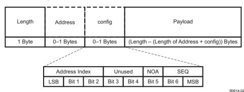
Figure 25-11. Structure of Packets in the Tx FIFO
