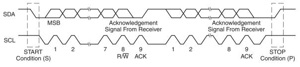
Figure 20-3. I<sup>2</sup>C Module Data Transfer
