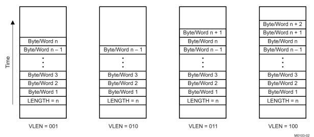
Figure 8-2. Variable Length (VLEN) Transfer Options
