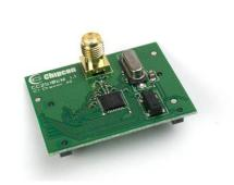
CC2430 Evaluation Module, a small plug-in module for CC2430DK. Should be used as reference design for antenna and RF layout.
