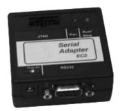
Figure 2: EC2 serial adapter
