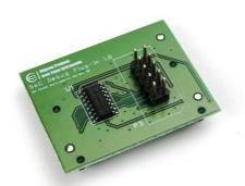
System-on-Chip debug plug-in module, a small plug-in module that should be used together with SmartRF®04EB when programming external target boards.
