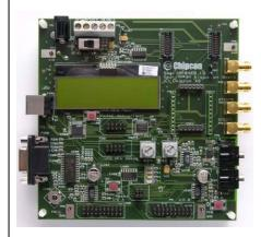
Evaluation Board. Main board with LCD, USB interface, LEDs, pot-meter etc. Platform for the Evaluation Modules (EM).
