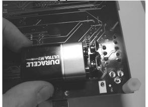
There are three different ways of applying power to the EB:
