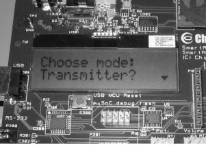
Select Transmitter on the other EB by moving the joystick. Confirm by pressing button S1.
