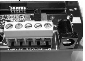
The second method applies DC power using the DC input jack (right in picture, centre is +, sleeve is ground), or by connecting a 4-10V voltage source between the 4-10V and 0V terminals of the power connector (left in picture). It is also possible to connect a 3.3V voltage source between the 3.3V and 0V terminals. The on-board voltage regulators will be bypassed in this case.
