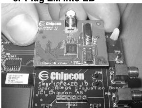
Insert a CC1110EM into both SmartRF04EBs. The connectors will only fit in one position, so that the EM cannot be inserted the wrong way. Do not force the EM.
