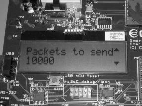
On the transmitter EB, select the number of packets to send. More packets takes longer but gives a better statistical result. Confirm by pressing button S1.
