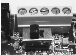
If a 3.3V source is used as described in 4b above, the switch should be set to the leftmost position. For all other cases, the switch should be set to the rightmost position. This switch can be used to turn off the EB by switching it to the opposite position of that used to turn it on.
