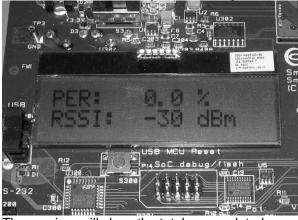
The receiver will show the total accumulated packet error rate together with the average signal strength (RSSI) of the previous 50 received
