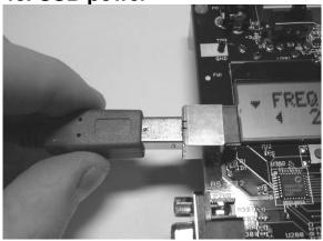
The EB can also be powered from the USB bus. Make sure that the SmartRF<sup>®</sup> Studio software is installed before connecting the EB to the PC, otherwise you may experience problems in installing it later due to driver issues.
