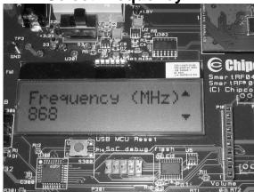
Select frequency according to the type of EM module in use (315 MHz, 433 MHz, 868 or 915 MHz). Move the joystick up or down to display the choices and push button S1 in the lower right corner of the board to select the displayed frequency.
