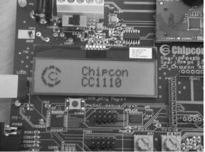
When power is applied to the board, the test program will start. You should see the Chipcon logo shown above on the LCD display on both EBs. Pushing button S1 in the lower right corner of the board will show the first menu item.
