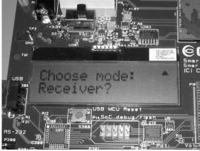
Select Receiver on the first EB by moving the joystick. Confirm by pressing button S1. The Receiving node will display "Ready to receive".
