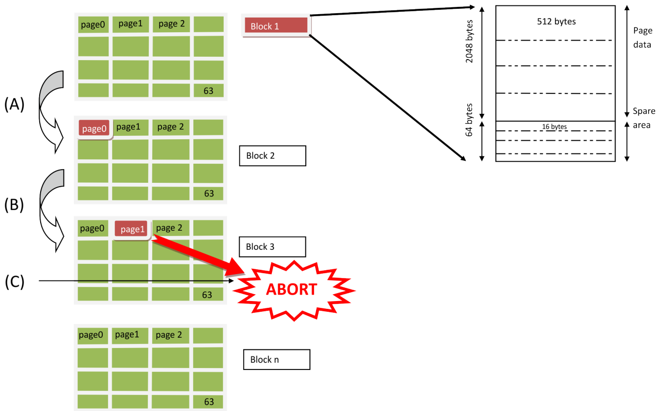
Figure 9. D800K008 ROM Behavior Before Application of Software Patch (1)
