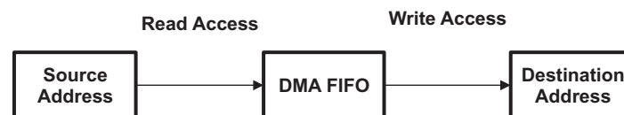
Figure 3-3. Two-Part DMA Transfer
