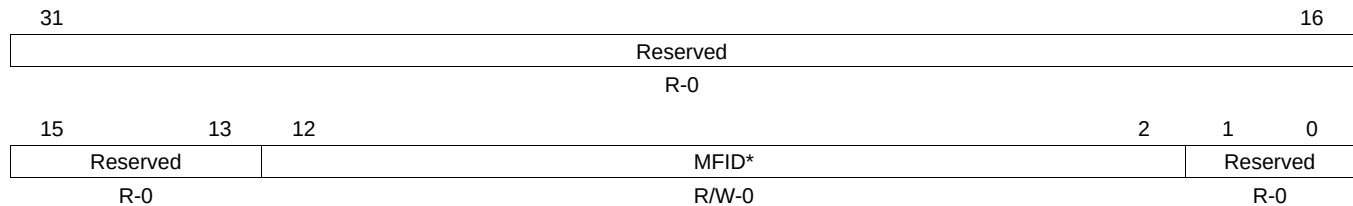
Figure 26-153. FIFO Rejection Filter Mask Register (FRFM) [offset_CC = 308h]
