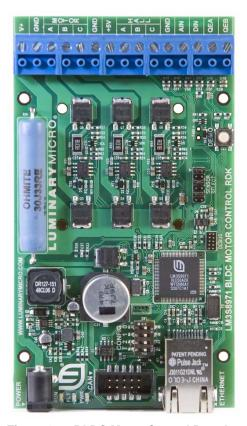
Figure 1. BLDC Motor Control Board
