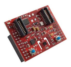
Plug-in BoosterPacks for the Tiva C Series TM4C123x LaunchPad make it simple and fun to explore various applications by expanding the functionality of the TM4C123G MCU.
