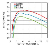
Figure 2. Conversion Efficiency Versus Output Current
