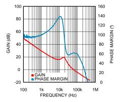
Figure 8. Open Loop Bode Response
