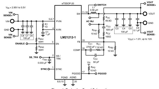
Figure 1. Evaluation Board Schematic
