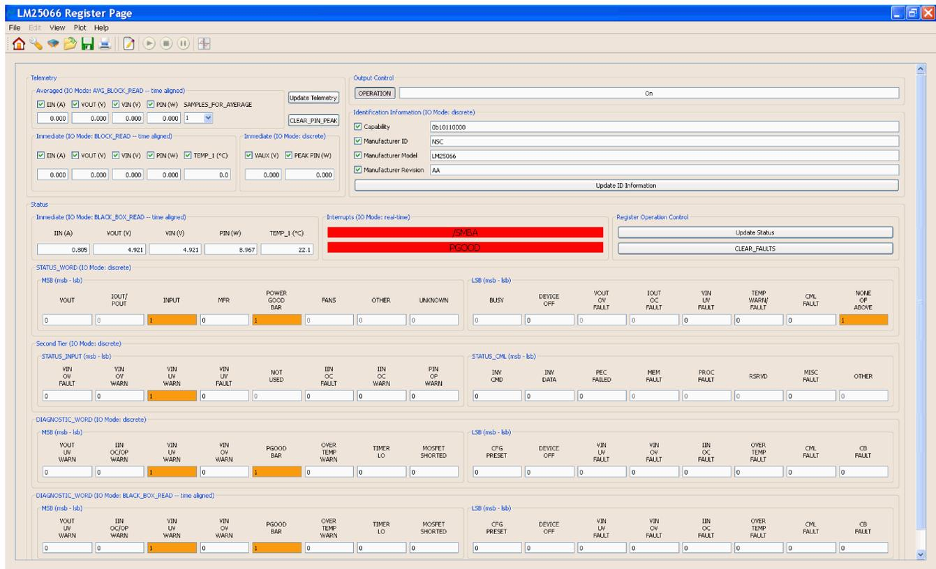
Figure 10. LM25066 GUI Register Page
