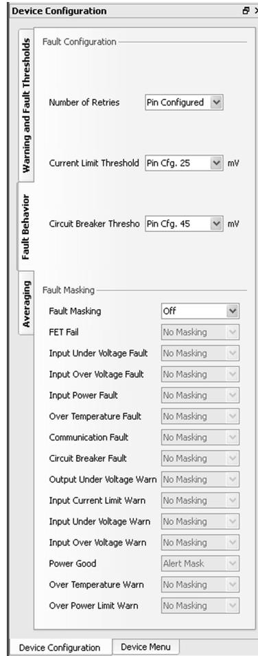
**Figure 8. Device Configuration Panel - Fault Behavior Tab**
