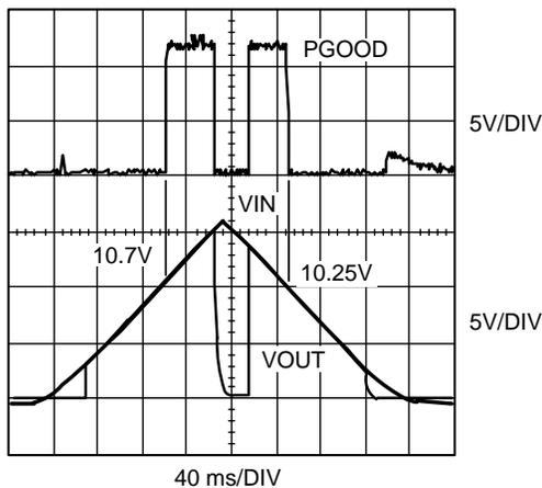
Figure 19. PGD Power up/Power down Behavior
