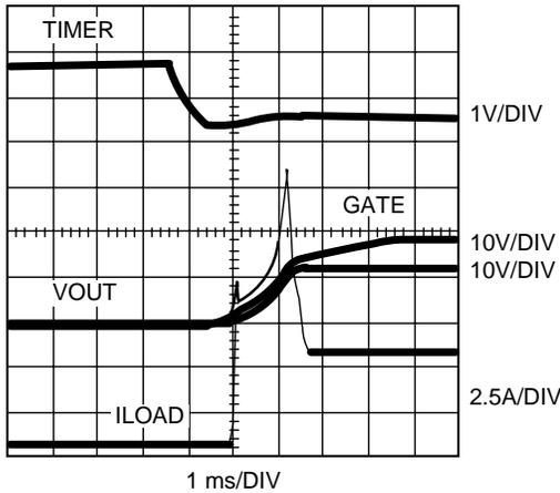
Figure 17. Turn-On Sequence into a 4Ω Load
