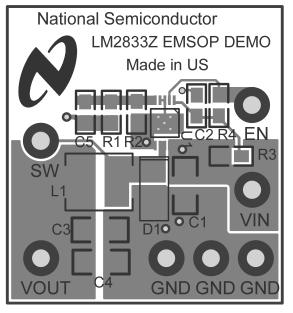
Figure 2. Top Layer and Top Overlay
