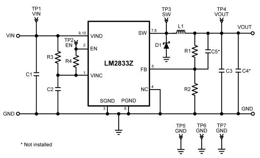
Figure 1. LM2833Z MSOP-PowerPAD Demo Board Schematic
