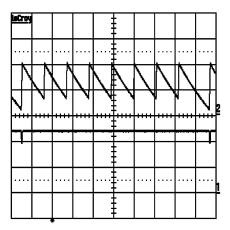
Horizontal Resolution: 2sec/div Trace 2: TIMER Pin, 2V/div Trace 1 Vout, 20V/div Vin = -48V, Ct = 2.2  $\mu$ F Voltages are respect to VEE
