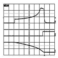
Horizontal Resolution: 0.5 ms/div Trace 4: Input Current, 2A/div Trace 2: PGD Pin, 50V/div Trace 1: Vout, 20V/div Vin = -36V
