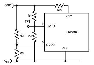
Figure 6. UVLO, OVLO Inputs (Option B)
