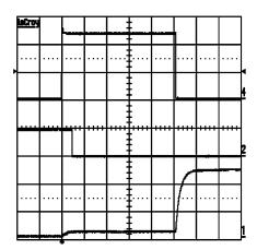
Horizontal Resolution: 20 ms/div Trace 4: Load Current 0 to 5A, 2A/div
