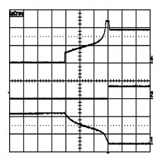
Horizontal Resolution: 5 ms/div Trace 4: Input Current, 2A/div Trace 2: PGD Pin, 50V/div Trace 1: Vout, 20V/div
