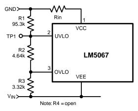
Figure 5. UVLO, OVLO Inputs (Option A)
