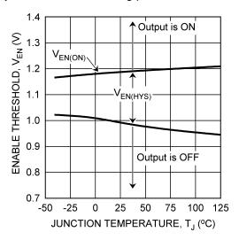
Figure 2. Enable Threshold
