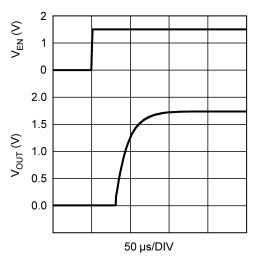
Figure 1.  $V_{OUT}$  vs.  $V_{EN}$
