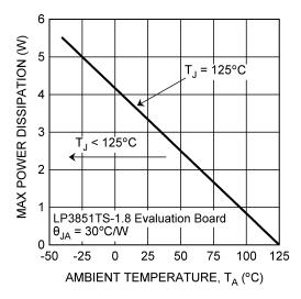
Figure 3. Maximum Power Dissipation vs. Ambient Temperature
