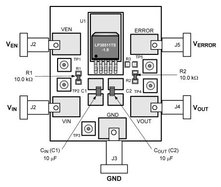
Figure 7. Evaluation Board Component and Pin Layout
