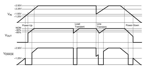
Figure 5.  $\overline{\text{ERROR}}$  Flag when Pull-Up is from  $V_{IN}$
