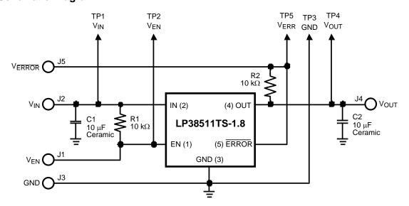
Figure 6. Evaluation Board Schematic
