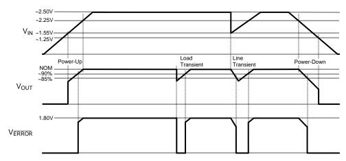
Figure 4. ERROR Flag when Pull-Up is from Vout
