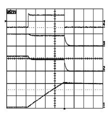
$\begin{array}{l} \mbox{Horizontal Resolution: 10 ms/div} \\ \mbox{Trace 1: TIMER Pin, 2V/div} \\ \mbox{Trace 2: GATE Pin, 50V/div} \\ \mbox{Trace 3: Vout, 50V/div} \\ \mbox{Trace 4: Input Current, 5A/div} \\ \mbox{Ct = 0.82 } \mu F \\ \mbox{V}_{IN} = 48V \\ \end{array}$
