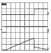
Horizontal Resolution: 100 ms/div Trace 1: TIMER Pin, 2V/div Trace 2: Vin, 50V/div Trace 3: Vout, 50V/div Ct = 0.82 µF
