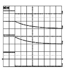
$\begin{array}{l} \mbox{Horizontal Resolution: 2 ms/div} \\ \mbox{Trace 1: UVLO Pin, 2V/div} \\ \mbox{Trace 2: GATE Pin, 50V/div} \\ \mbox{Trace 3: Vout, 50V/div} \\ \mbox{Trace 4: Input Current, 5A/div} \\ \mbox{V}_{\rm IN} = 48V \end{array}$
