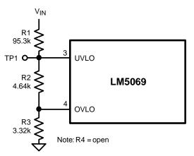
Figure 5. UVLO, OVLO Inputs (Option A)
