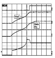
$\begin{array}{l} \mbox{Horizontal Resolution: 2 ms/div} \\ \mbox{Trace 1: GATE Pin, 20V/div} \\ \mbox{Trace 2: PGOOD Pin, 50V/div} \\ \mbox{Trace 3: Vout, 20V/div} \\ \mbox{Trace 4: Input Current, 2A/div} \\ \mbox{V}_{\rm IN} = 36V \end{array}$
