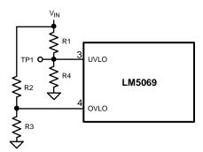
Figure 6. UVLO, OVLO Inputs (Option B)
