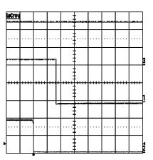
Horizontal Resolution: 5 µs/div Trace 1: PGOOD Pin, 20V/div Trace 2: UVLO Pin, 2V/div Trace 3: Vout, 20V/div
