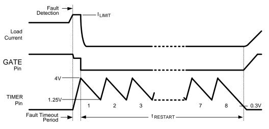
Figure 4. Fault Timeout and Restart Sequence
