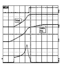
$\begin{array}{l} \mbox{Horizontal Resolution: 1 ms/div} \\ \mbox{Trace 1: GATE Pin, 20V/div} \\ \mbox{Trace 2: PGOOD Pin, 50V/div} \\ \mbox{Trace 3: Vout, 20V/div} \\ \mbox{Trace 4: Input Current, 2A/div} \\ \mbox{V}_{\rm IN} = 36V \end{array}$
