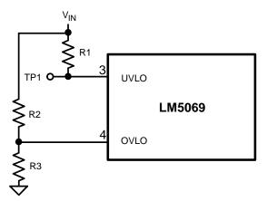
Figure 7. Minimum UVLO Threshold, Adjustable OVLO
