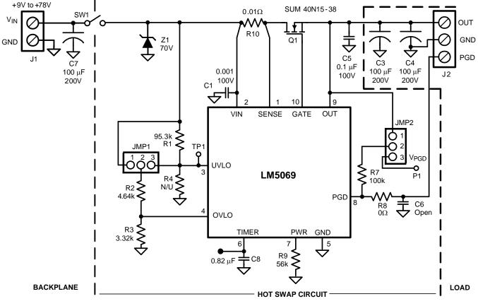
The LM5069EVB is supplied with pins 2-3 jumpered on JMP1, and pins 1-2 jumpered on JMP2.
