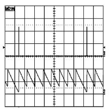
$$\label{eq:horizontal Resolution: 1s/div} \begin{split} & \text{Horizontal Resolution: 1s/div} \\ & \text{Trace 2: TIMER Pin, 2V/div} \\ & \text{Trace 3: Vout, 5V/div} \\ & \text{Ct} = 0.82 \ \mu\text{F} \end{split}$$
