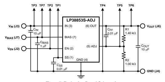
Figure 7. Evaluation Board Schematic.
