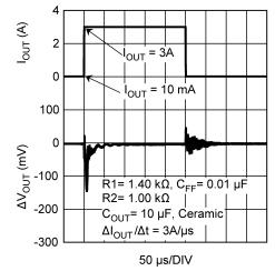
Figure 1. 10mA to 3A Load Transient Response
