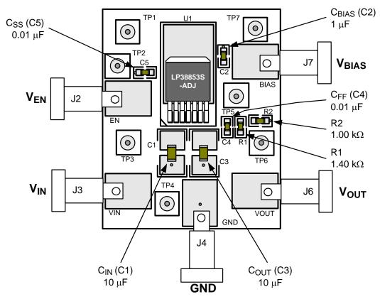
Figure 8. Evaluation Board Component and Pin Layout
