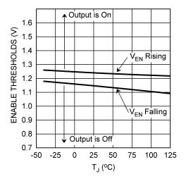
Figure 3. Enable Thresholds
