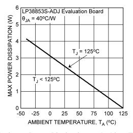
Figure 5. Maximum Power Dissipation vs Ambient Temperature
