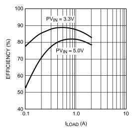
Figure 3. LM2852X Typical Efficiency for 2.5 V Output
