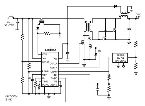
Figure 1. Simplified Active Clamp Forward Converter
