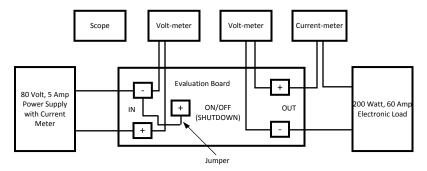
Figure 2. Typical Evaluation Setup
