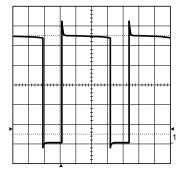
Figure 7. Drain Voltage
