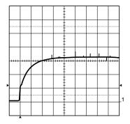
Figure 3. Output Voltage During Typical Startup
