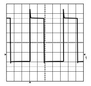
Figure 6. Drain Voltage
