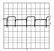
Figure 8. Gate Voltages of the Synchronous Rectifiers
