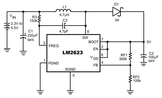
Figure 1. Evaluation Board Application Circuit
