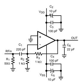
Figure 4. Coupling the RF Signal to the IN- Pin Circuit Diagram
