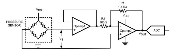
Figure 10. Pressure Sensor Application
