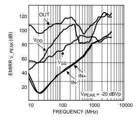
Figure 7. EMIRR vs. Frequency for IN+, IN-, V<sub>DD</sub>, V<sub>SS</sub>, and OUT
