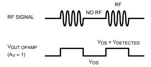
Figure 1. Offset Voltage Variation Due to a Detected RF Signal
