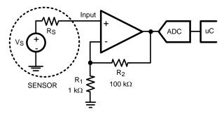
Figure 9. Typical Signal Path Application
