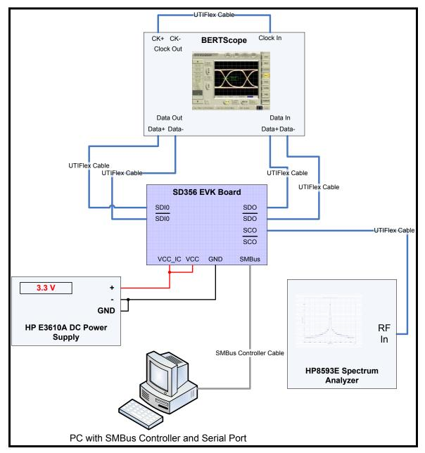
Figure 2. Test setup for the SD356EVK board.
