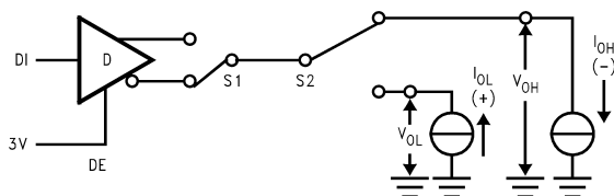
Figure 4. Driver V_{OH} and V_{OL}
