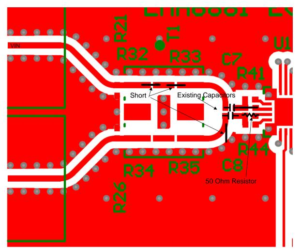
Figure 4. Input Configuration for Single Ended Signal. R44 should be 50 $\Omega$  to ground. R32, 33 are 0 $\Omega$  shorts. R34 and R35 are not needed.
