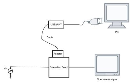
Figure 6. Typical Bench Setup
