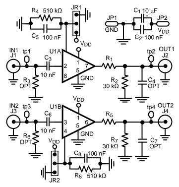
Figure 1. Schematic of the Evaluation Board
