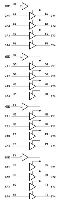
LOGIC DIAGRAM (POSITIVE LOGIC)
